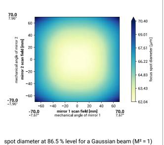
spot diameter at 86.5% level for a Gaussian beam ( $M^2 = 1$ ) with 8.0 mm diameter at  $1/e^2$ , clipped at 8.0 mm field size and mirror distances as given above for a two mirror scan system
